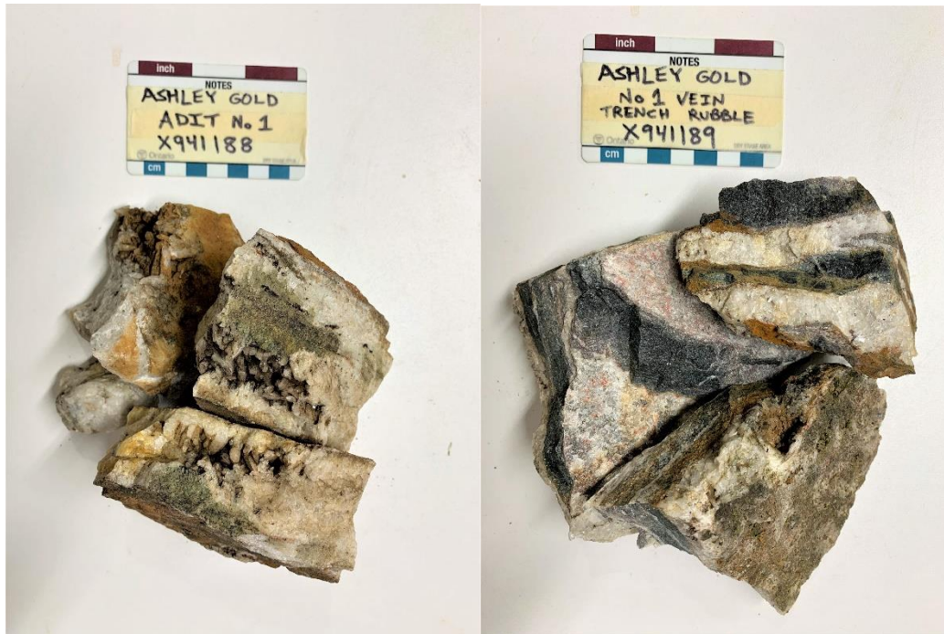
FIGURE 18: SAMPLE PHOTOS OF VEIN NO.1 AND ALTERED BASALT HOST
