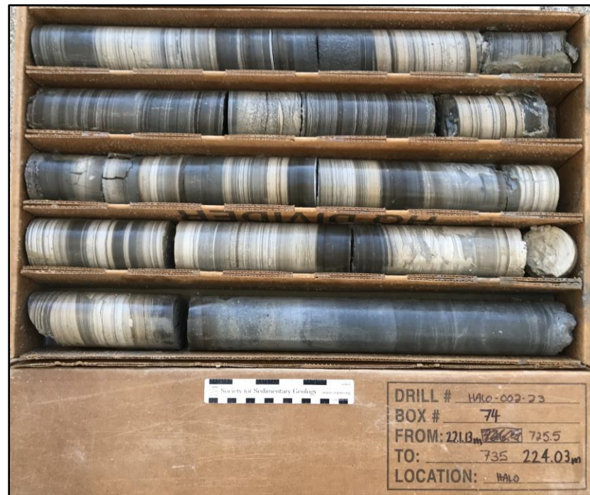
Figure 2. Finely laminated claystone at 221.13 to 224.03 metres, Drill Hole No. HALO-002-23.
