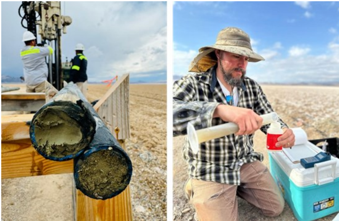
Image 2: Sampling sleeves and material from the top ten feet of Geoprobe hole CB24-013G (left).
