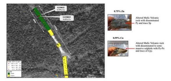
Figure B: T22:01 Trenching Details
