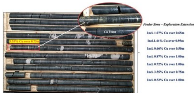
Figure 2: Chester Core Hole ID: C21-07: Copper Stringer Zone Extension (CNW Group/Canadian Copper Inc.)
