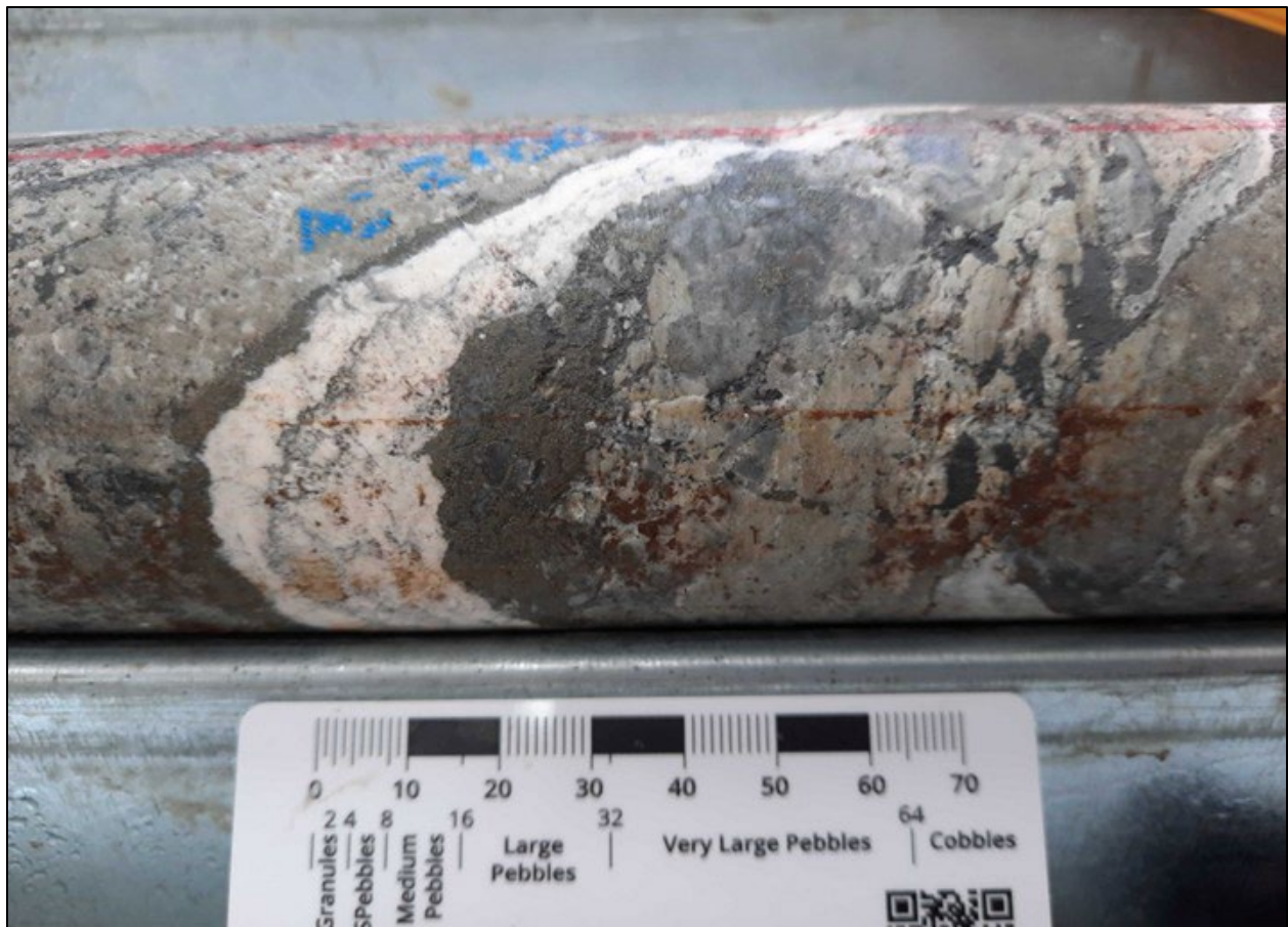
Figure 2. Carbonate base metal vein registering 2,100 ppm arsenic by pXRF ( click here to view image ).
