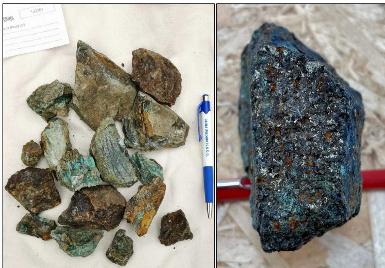
Figure 3. Macroscopically observed copper mineralization in samples 103281 and 103276 which returned 1.45 % and 2.47 % Cu, respectively. Mineralization is vein-hosted within potassic altered diorites and comprises quartz, chalcopyrite, malachite, azurite and tenorite ( click here to view image ).
