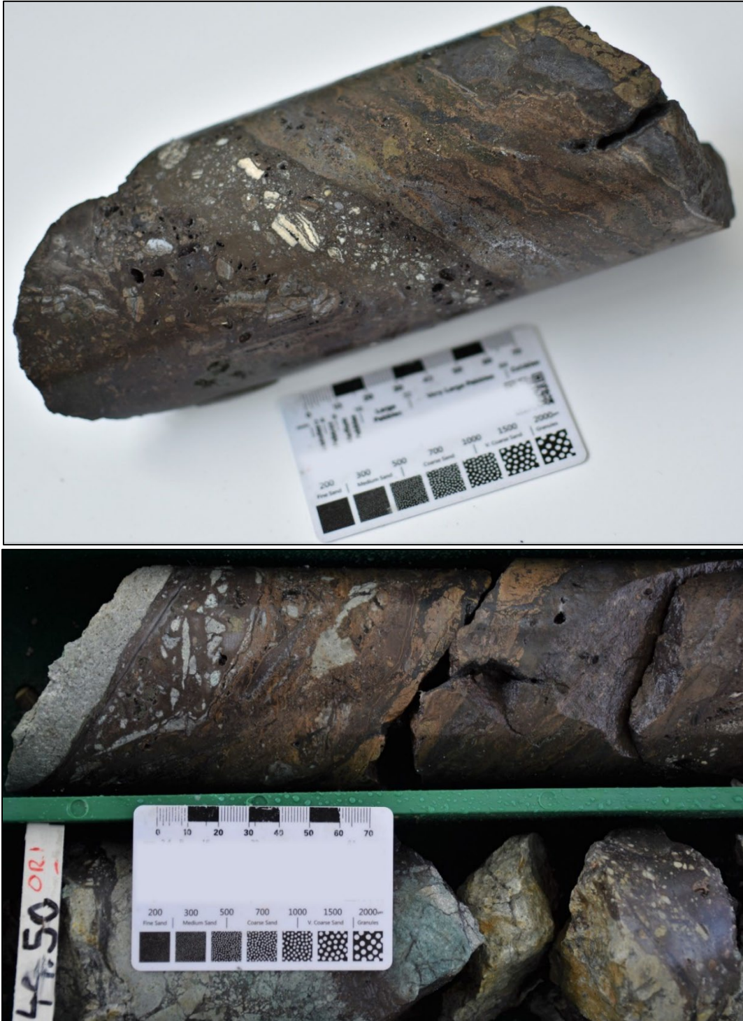
Figure 3. PQ3 diameter diamond drillhole CMV23003 illustrating intervals of colloform banded orange-brown sphalerite and galena, including sections of hydrothermal breccia and a sharp upper vein contact with the argillic altered andesitic tuffaceous breccia. Coarse grained sulphides are present between the colloform bands ( click here to view image ).
