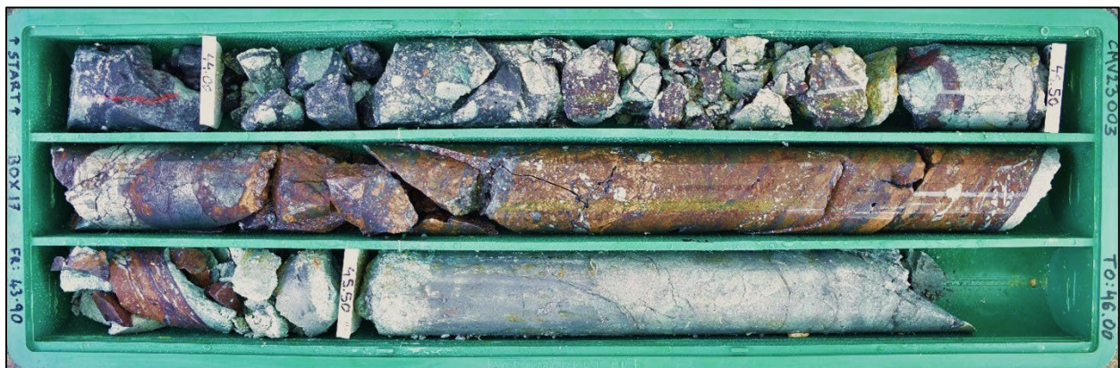
Figure 2. Massive sulphide interval between 43.90-46.00 m downhole in CMV23003. 44.60-45.50 m hosts massive colloform banded orange-brown sphalerite and galena with intervals of hydrothermal brecciation, which grades downhole from an andesitic volcanic breccia which has been completely matrix replaced by a polymetallic sulphide assemblage ( click here to view image ).
