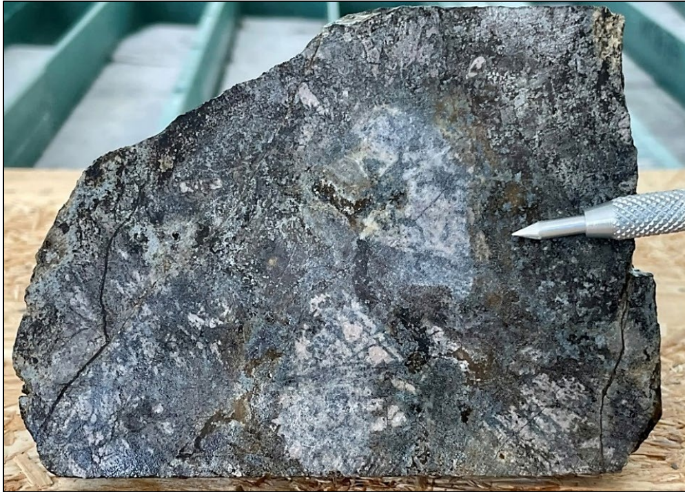
Figure 4. Retrograde skarn with sphalerite-chalcopyrite at 37.5 m (2.74 g/t Au). ( Click here to view image )
