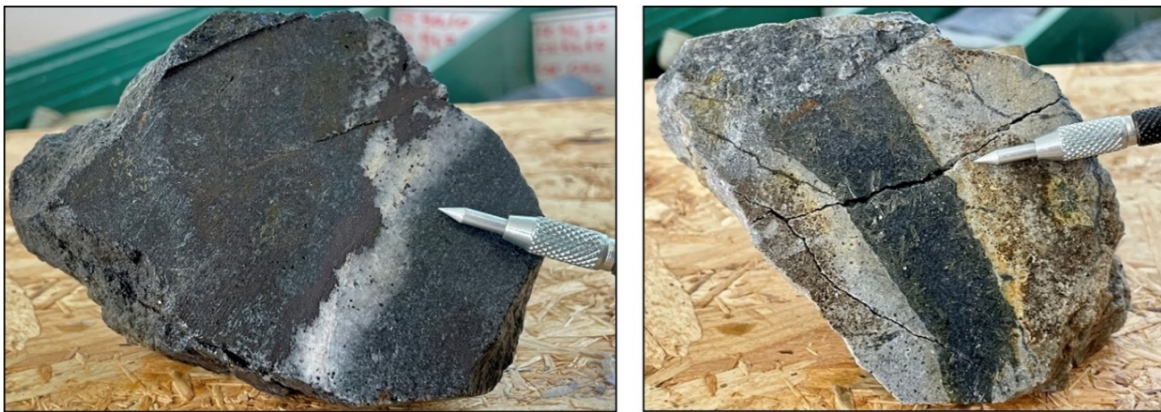
Figure 5. Drill core from CMVDD004 illustrating both semi-massive sulphides and a footwall vein of quartz-carbonate-sulphide. Sulphide assemblage dominated by sphalerite with marcasite, jamesonite and silver-bearing sulfosalt freibergite with trace miargyrite (2 cm scratcher tip; click here to view image ).
