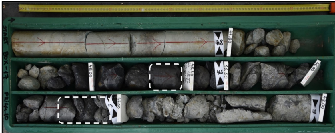
Figure 4. Drill hole CMVDD004 between 44.1 m and 48.0 m. Footwall veins and semi-massive sulphide intervals can be observed. Figure 5 (below) is outlined by white rectangles ( click here to view image ).
