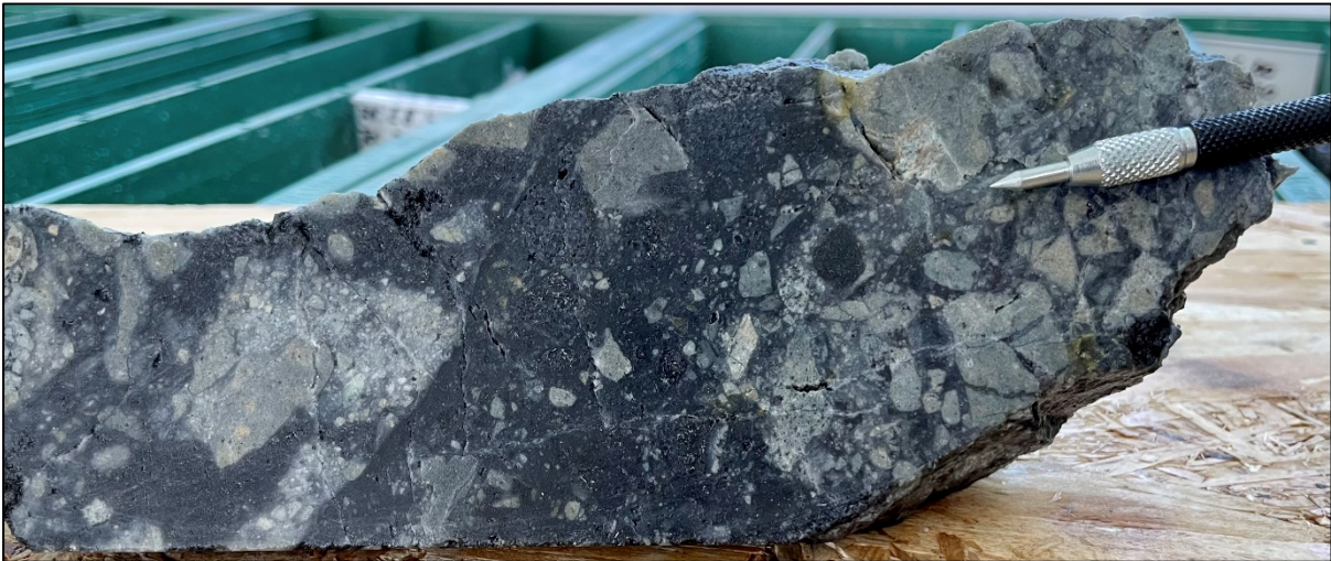
Figure 7. Drill core segment 87.15 – 87.45 m from CMVDD005. Sulphide-quartz cemented hydrothermal breccia with sub-angular clasts of silicified andesitic tuff host rock. Sulphide assemblage comprises stibnite-sphalerite-berthierite with trace inclusions of miargyrite. (2 cm scratcher tip for scale; click here to view image ).
