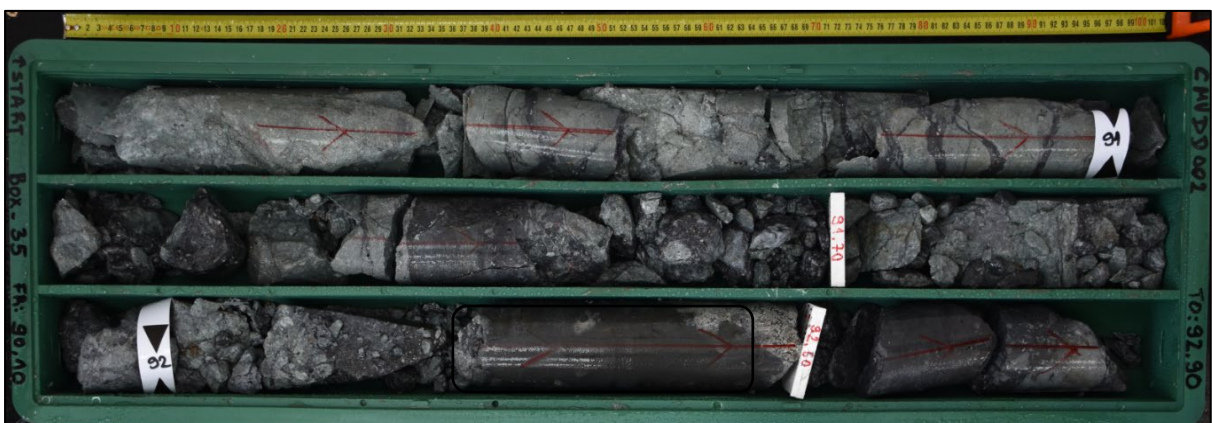
Figure 5. The CMVDD003 drill core from 90.1 to 92.9 m. Hanging wall stringers and semi-massive sulfide veins are observed. Details of the dashed rectangle are outlined in Figure 4. Click here to view image
