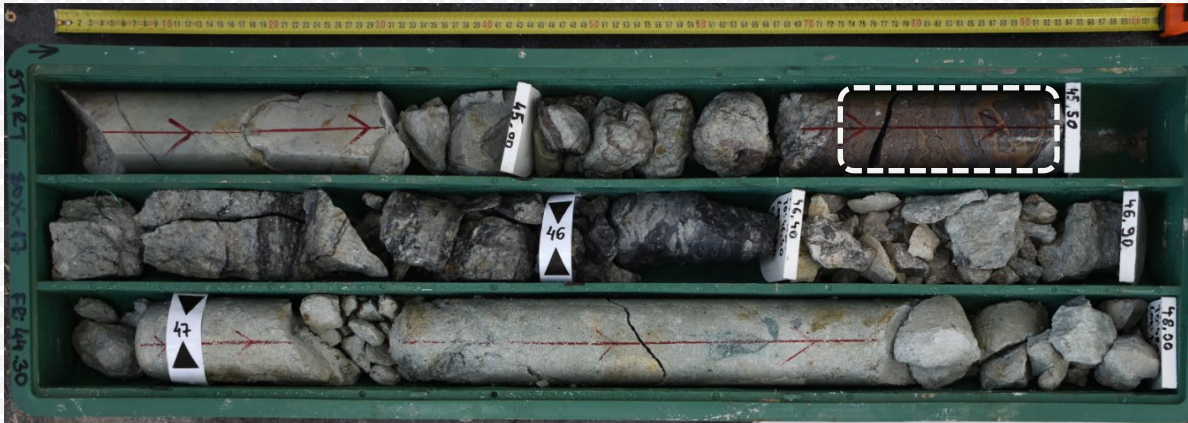
Figure 3. Photograph of 44.3 – 48.0 m in drillhole CMVDD002. Orange, brown colloform banded sphalerite can be observed with galena in polymetallic vein. Photo 2 is outlined by white rectangle. Click here to view image
