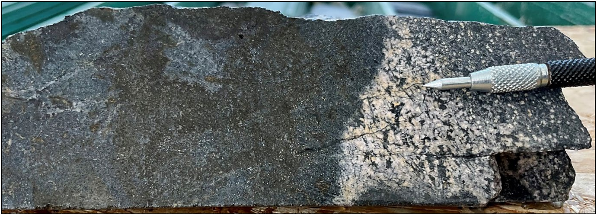
Figure 6. The CMVDD003 drill core segment from 92.4 to 92.6 m with semi-massive sphalerite-stibnite-galena-pyrite-pyrrhotite assemblage along the vein-tuff contact. Click here to view image
