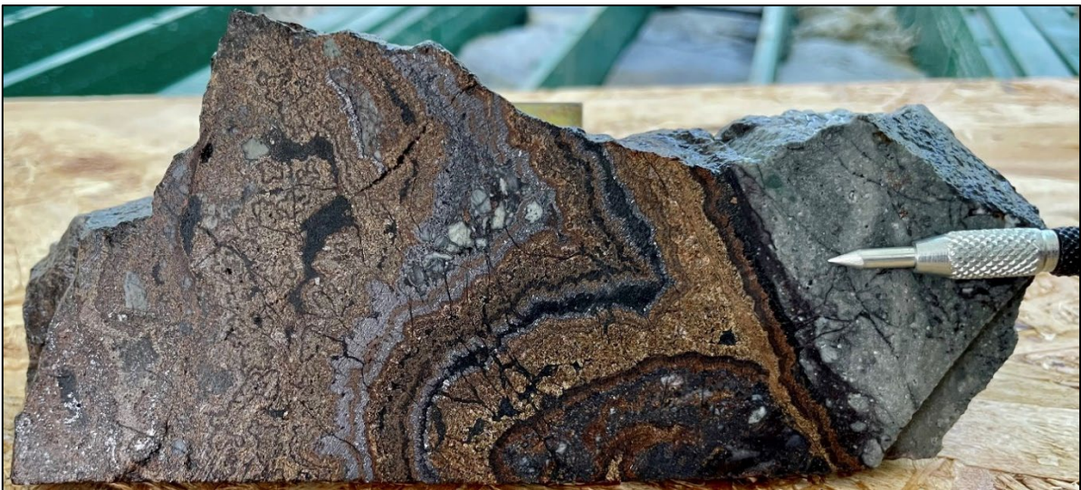
Figure 4. Photograph of 45.35 – 45.50 m in drillhole CMVDD002. Orange, brown colloform-crustiform banded sphalerite and galena can be observed with weakly brecciated lower vein contact with andesitic tuff. Click here to view image
