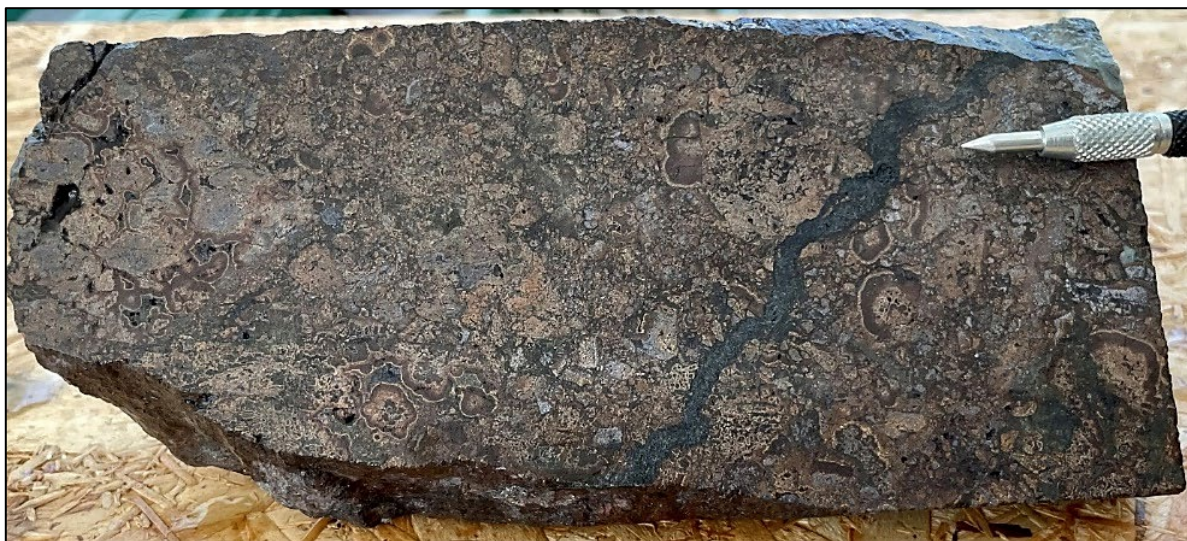
Figure 4. CMVDD001 interval from 30.8 to 31.0 m. Colloform banded sphalerite with galena aggregates cut by a sphalerite-stibnite-galena vein (2 cm scratcher tip for scale). Click here to view image.
