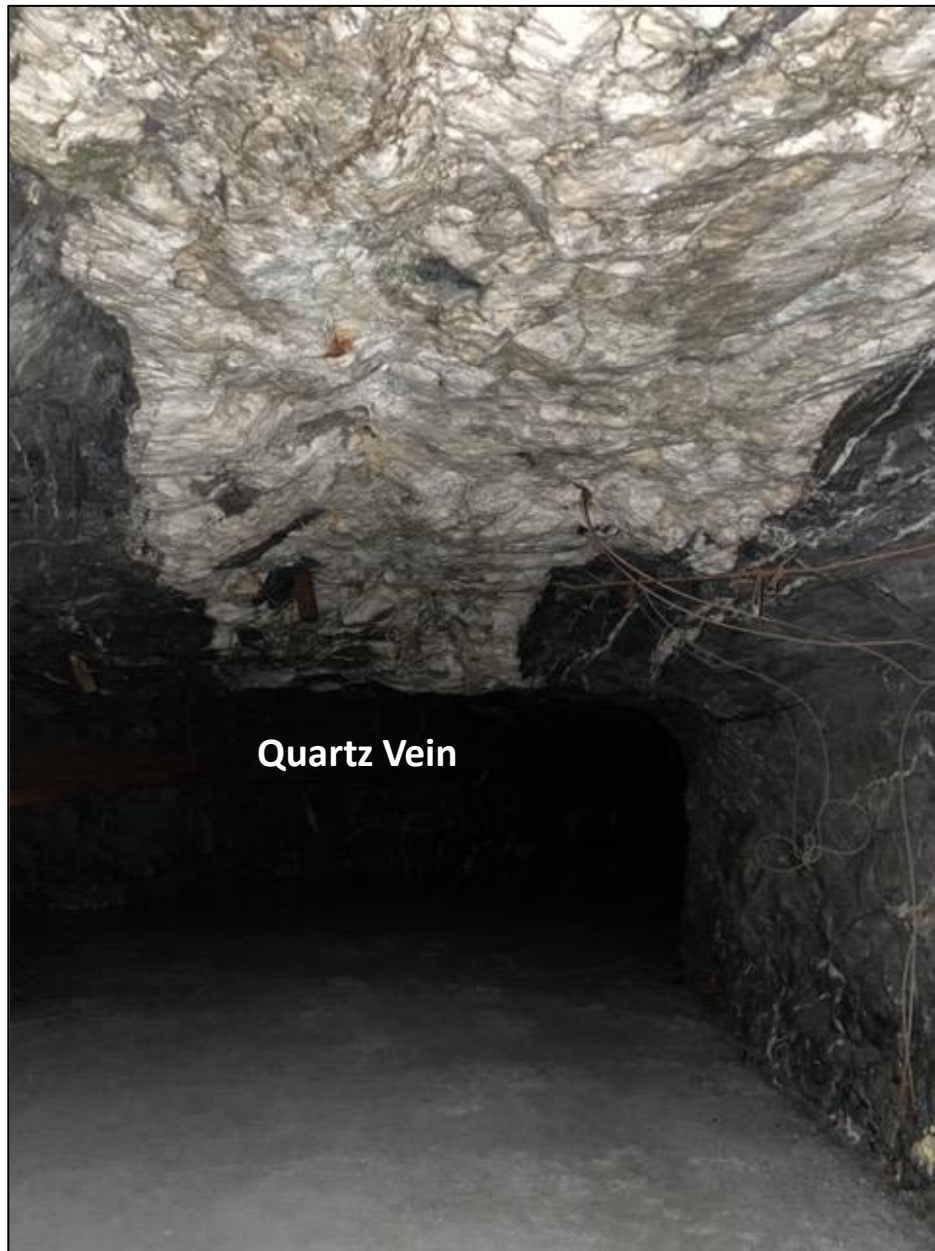
Photo 7 – Level 6950 3-meter Eagle quartz vein exposed on the back (roof) of the drift
