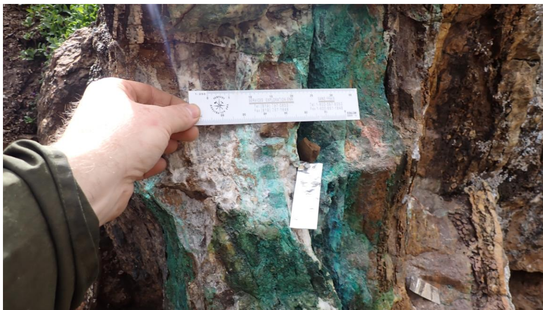
Float Sample D – 723409; 7.69% Copper, 49.80 g/t Ag, 1,761 meters elevation
