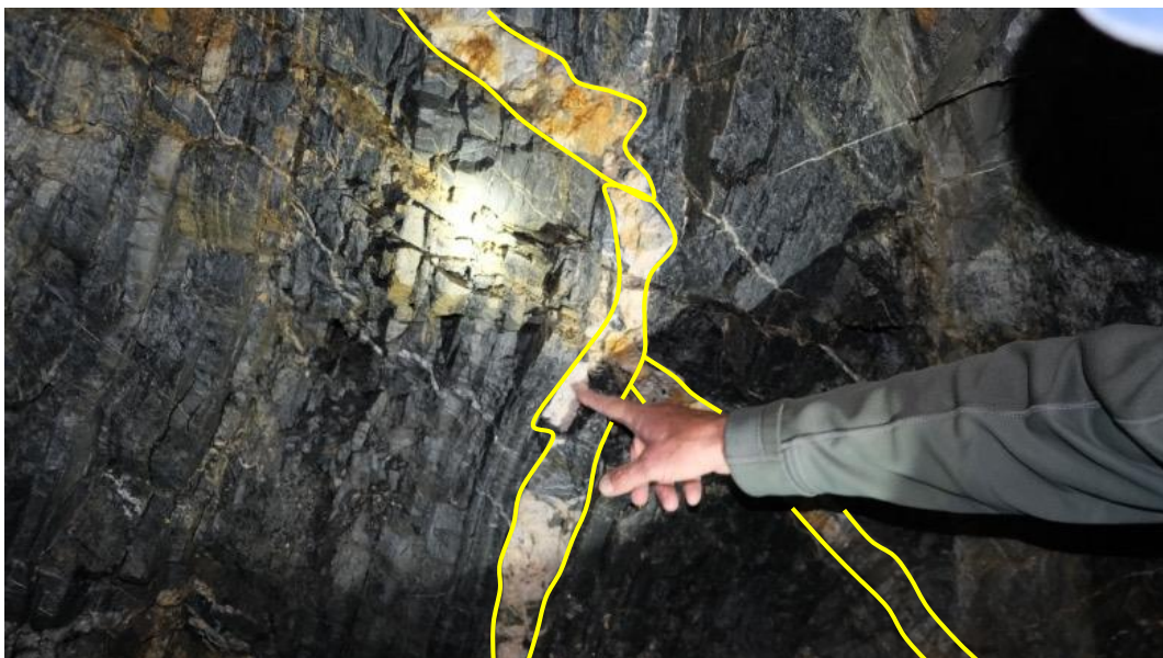
Underground Harris – close up tension fracturing healed with white quartz, note displacement
