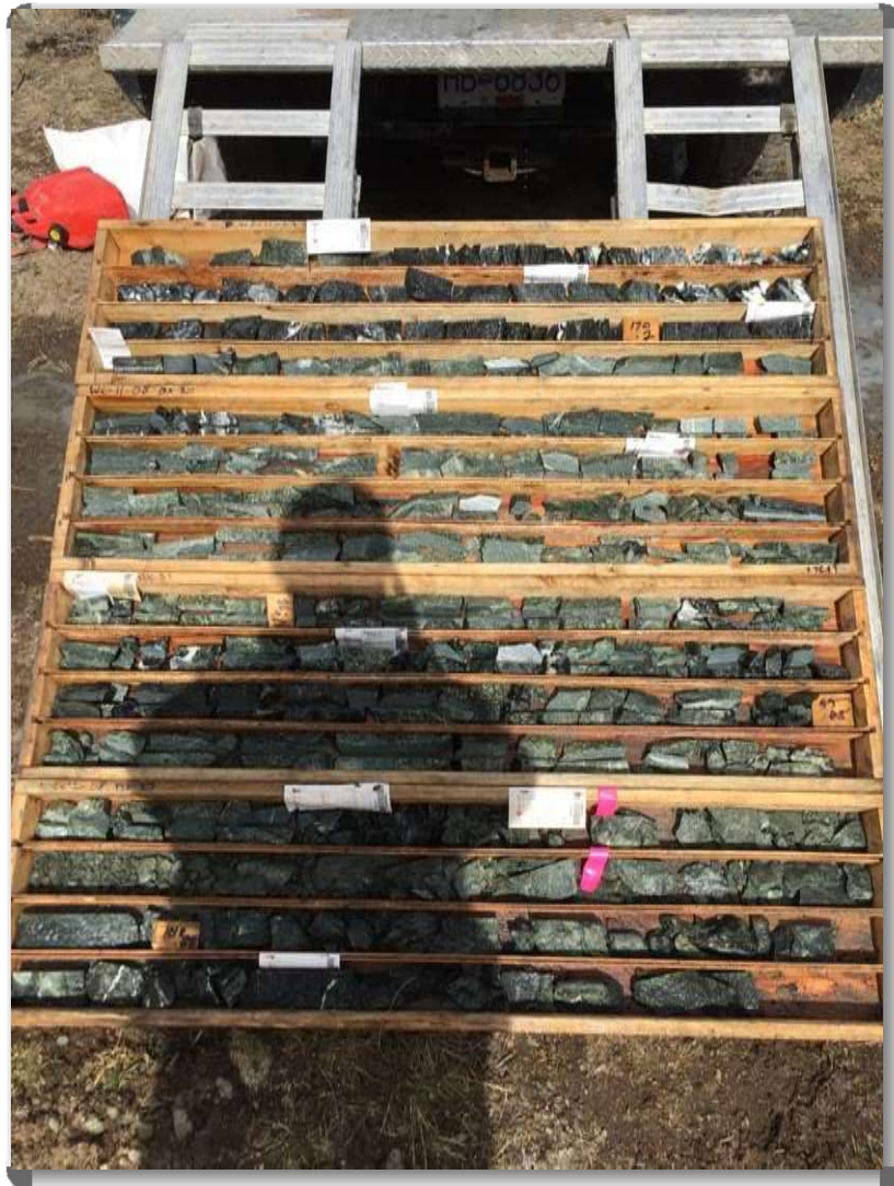
Figure 12.4: Data verification sampling - Picture showing quartered drill core which was subsequently sampled.
