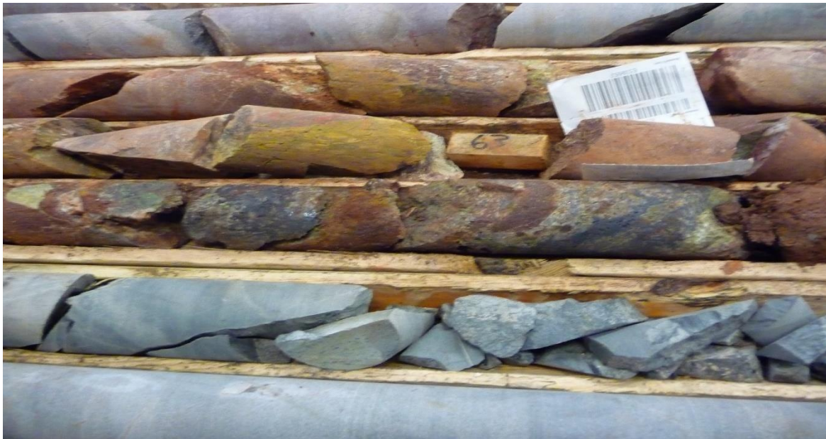
Photo 1: Chalcocite in Drill hole DL21-01. Note the blue grey chalcocite in the Center of the Photo.
