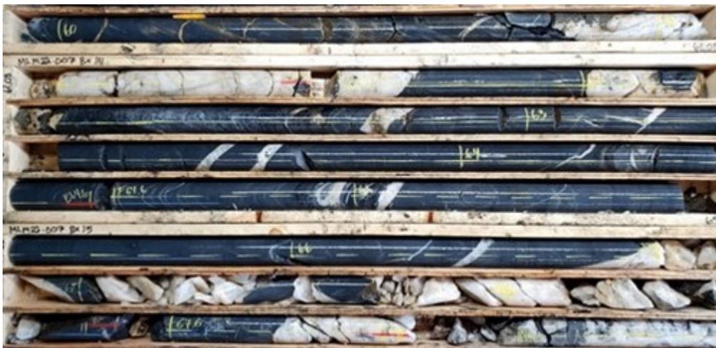
**Figure 2: MLM22-007 60-69m quartz veining. Pyrite stringers disseminated pyrite occasionally present. Host rock is metasediment.**
