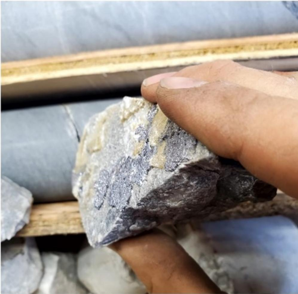
**Figure 3: Galena coating fractures from MLM22-05 at 102m**
