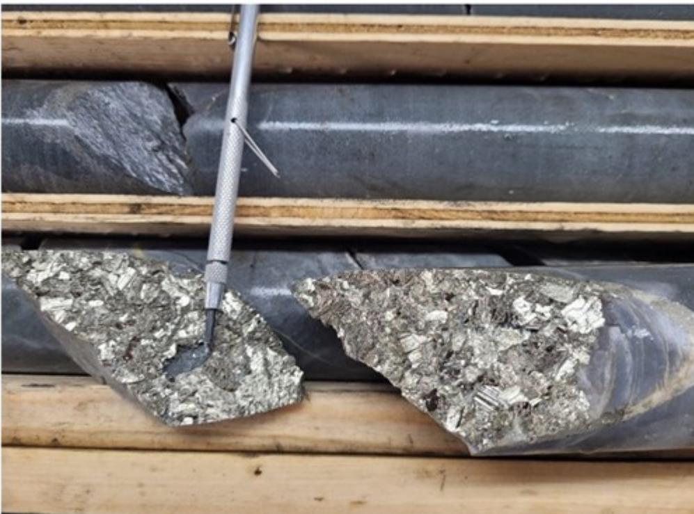
**Figure 4: Pyrite in siderite veins in hole MLM22-10**
