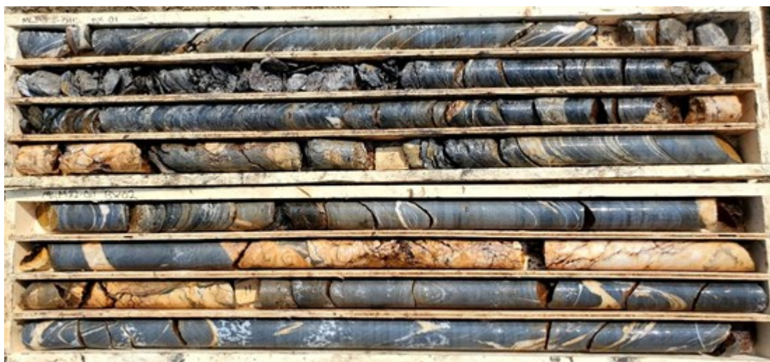
Figure 3. First two boxes of MLM22-011—Fractured vuggy quartz siderite vein with pyrite and sulfosalts, typical of Keno Hill Silver Mineralization (KHSM).
