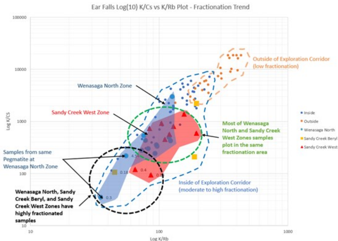
Figure 8 Log base 10 K/Cs Vs K/Rb Plot of Fractionation Intensity of Ear Falls Samples
