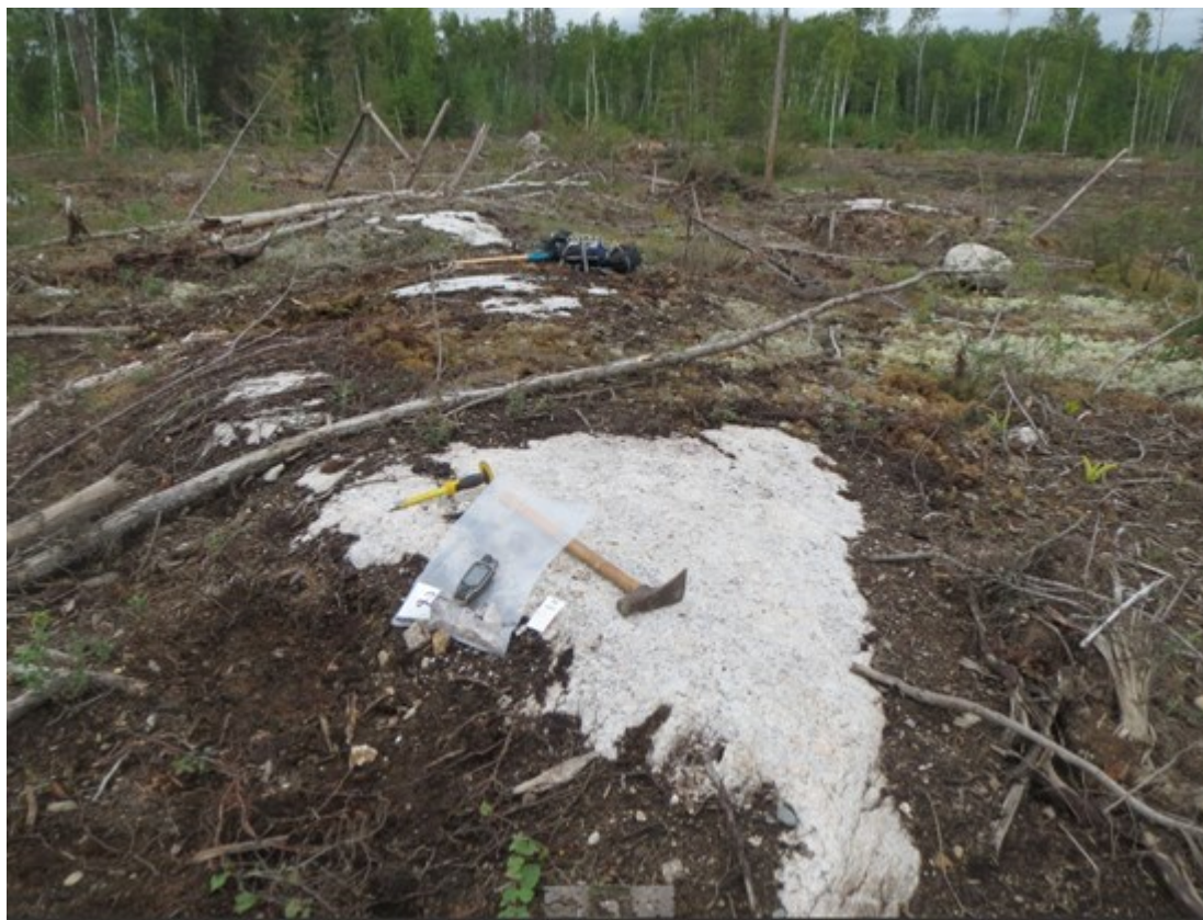
Figure 9 Pegmatite Identified in the Sandy Creek West Zone Located 7 KM SW of the Wenasaga North Zone with Grab Sample up to 0.40% Li 2 O
