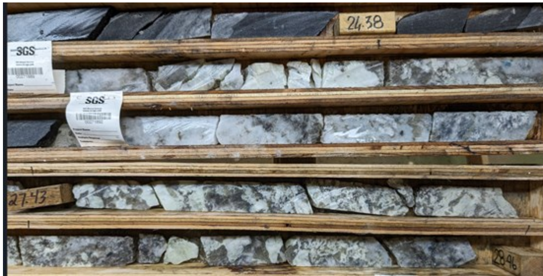
Figure 5 EF23-04 Drill Core Pic of Spodumene-bearing Pegmatite Intercepted at 25.16m at depth - Wenasaga North Zone
