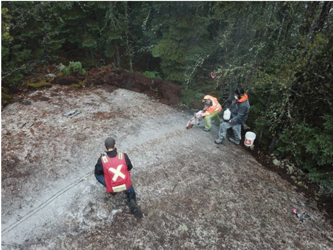
Figure 4 Field Crew Channel Sampling the Last Resort Pegmatite while Senior Prospector, Jace Angell, Making Field Note
