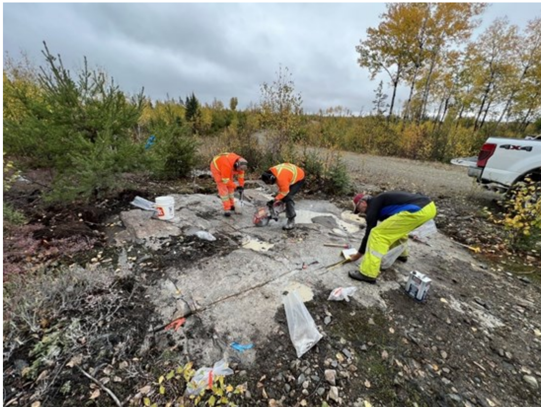
Figure 1 Paul Baxter, Beyond Lithium's Sr. Geo, measuring the width and mapping of the spodumene-bearing pegmatite along the main logging road at the Ear Falls Project with two Jr. Geo sampling the dyke.
