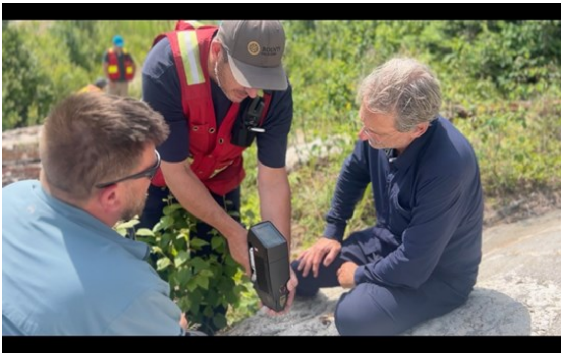
Figure 4: Senior Prospector Jason Leblanc utilizing the LIBS analyzer.
