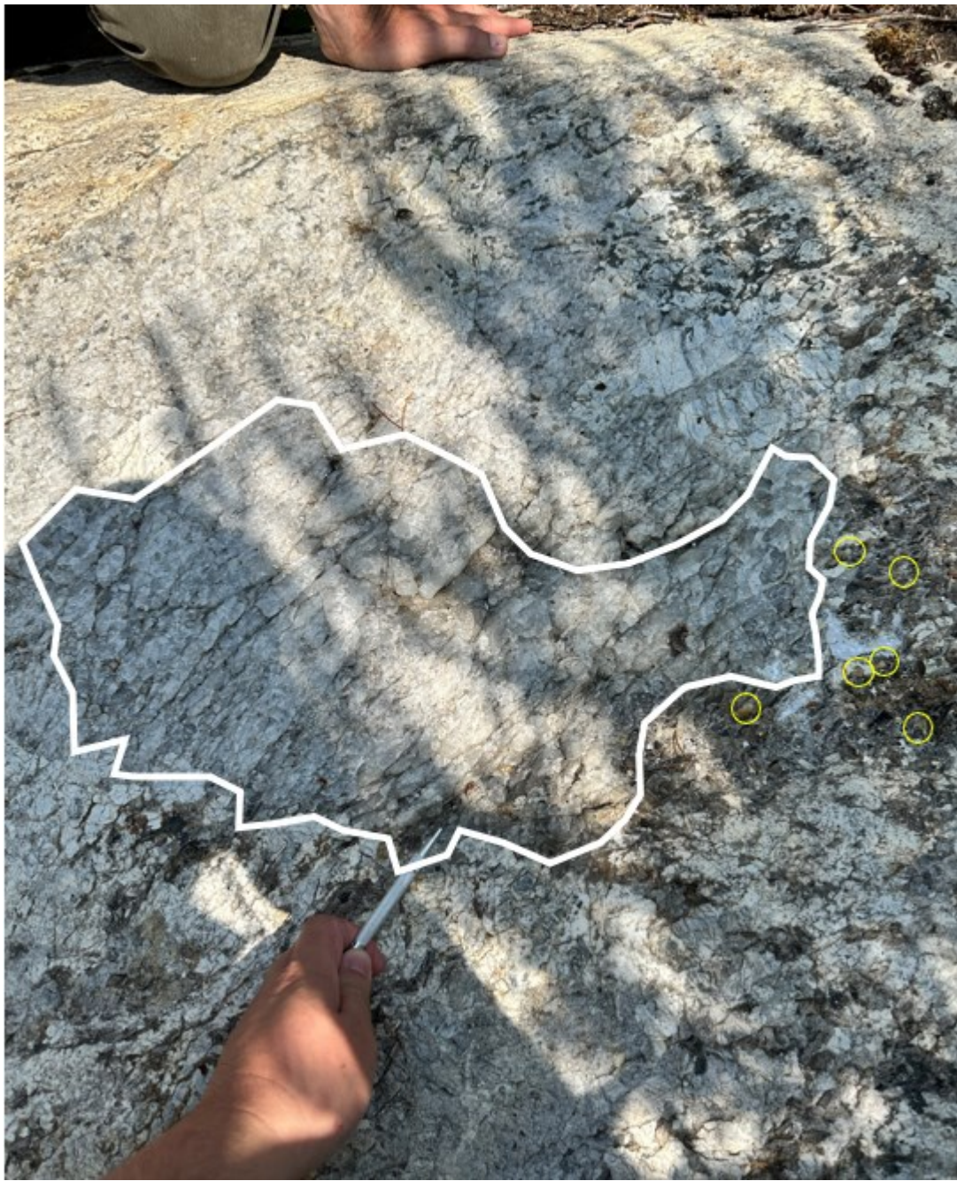
Figure 3: Example of Zoned Pegmatite with Beryl in Yellow Mineralized Around Larger Quartz in White crystal
