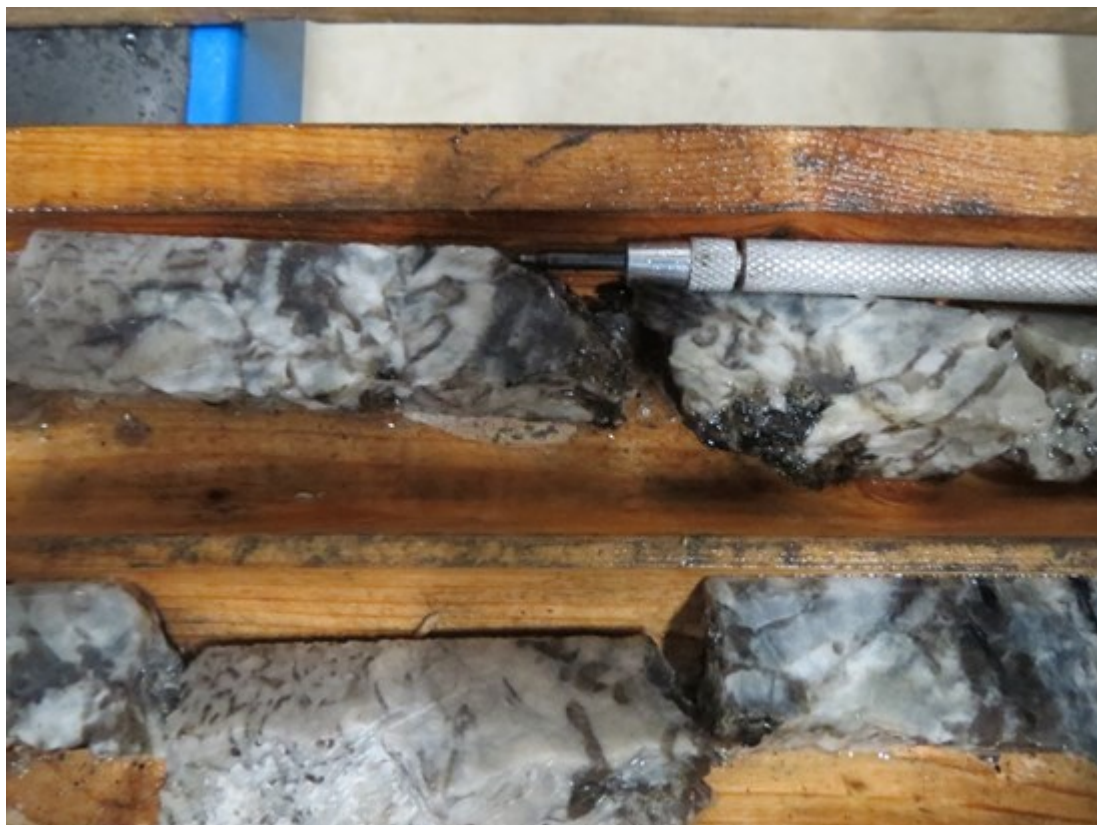
Figure 2: Muscovite-Biotite Pegmatite Dyke Recorded from 89.04 to 92.54m at depth from Historical Drill Hole MET-01 from the Sollas Lake Property
