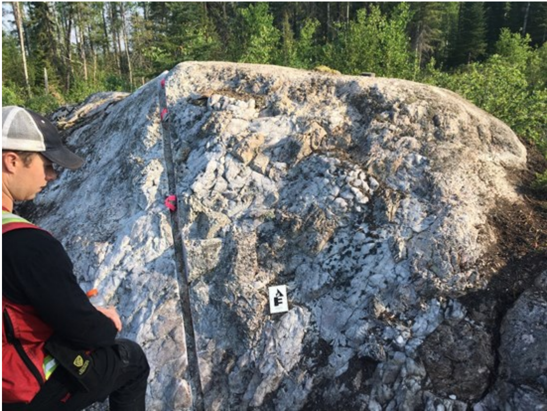
Figure 5: Field Crew Taking Notes of the Channel Sampled Beryl-Bearing Pegmatite Outcrop from the Cosgrave Lake Property
