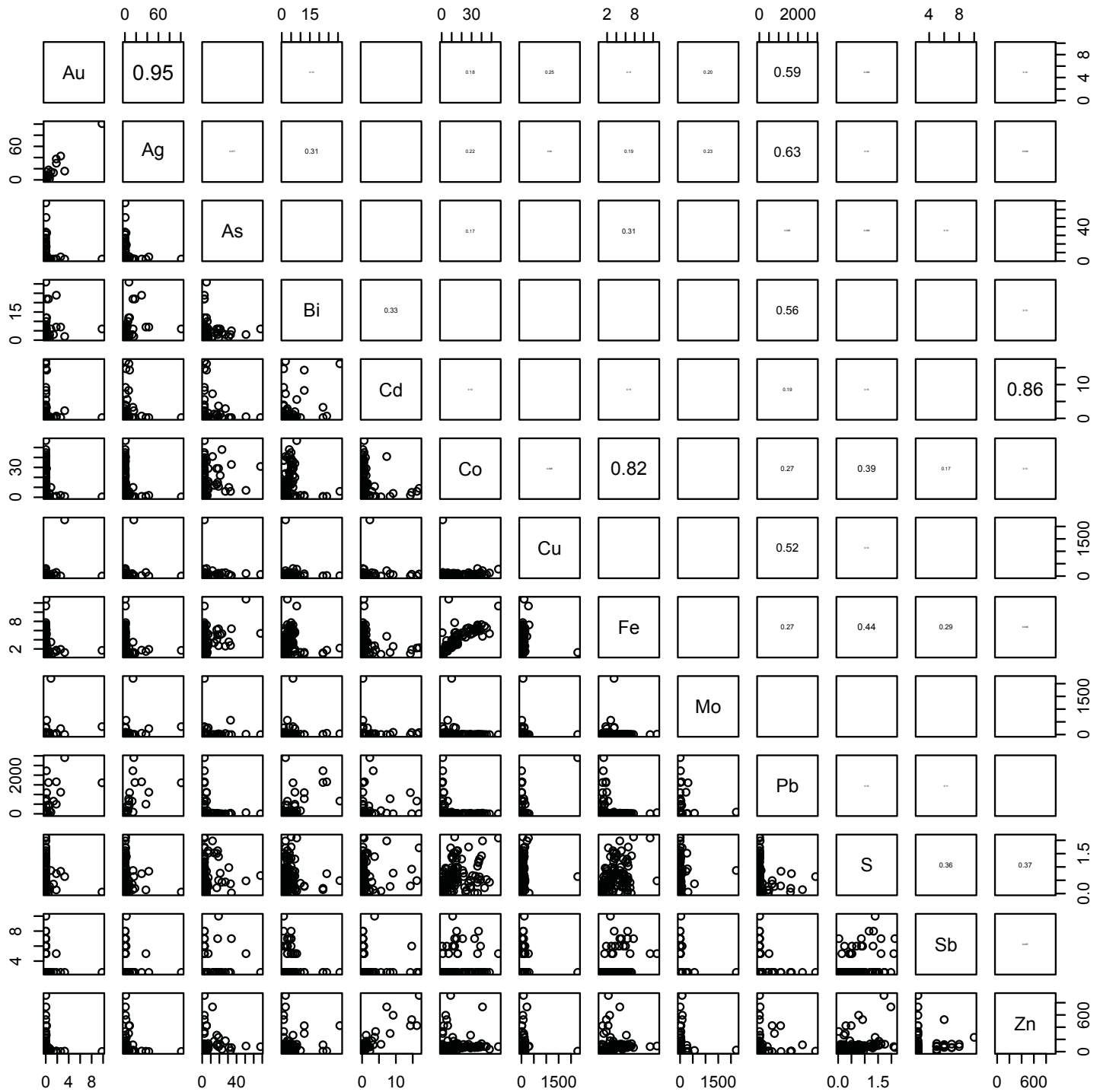
Figure 36: Element Correlation chart for the Chuchi South rock samples
