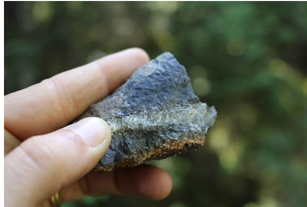
(B) Moderately chloritized and magnetized mafic rock with 3% sericite veinlets from outcrop near soil sample 2045908.
