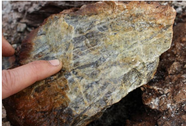
(B) Zoom on the host-rock in between quartz-sericite vein (A) with 10 ppb Au, 746 ppm As and 37 ppm Sb.
