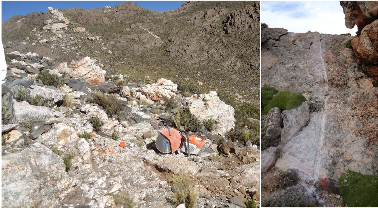
Figure 6: Example of channel sampling done by Rojas Mining Advisors for Centenera Mining Corporation during 2017 and 2018. A: General view of the grinder and pegmatites. B: Detail view on the channel.
