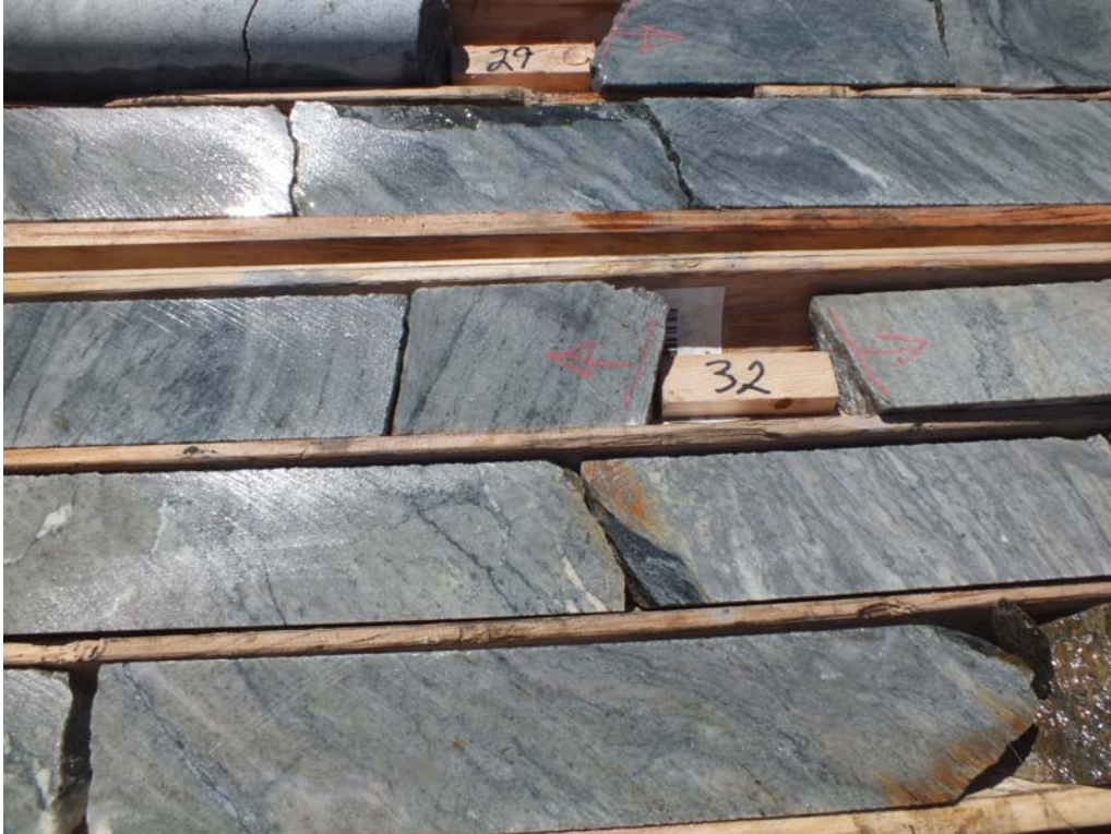
Figure 8. Core photo of silica-albite-ankerite-sericite gold zone in BE17-07 that returned 1.14 g/t Au over 5.9m from 32 to 37.9m.
