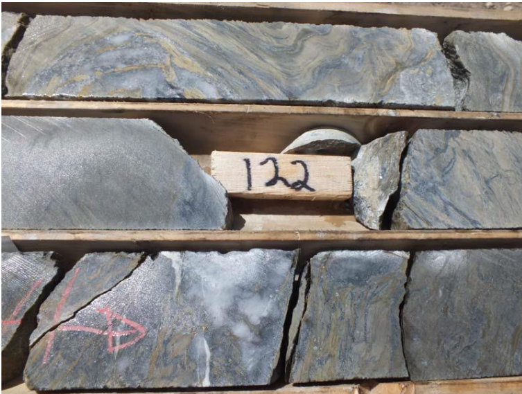
Figure 9. ore photo of the carbonate-sericite zone BE17-04 with an intercept of 0.298 g/t Au from 122.2 to 123.2m
