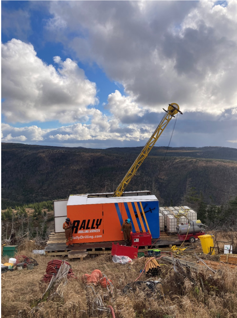
Photo 1: Diamond Drill Set up at Drill Hole GR-24-1 at Steep Brook
