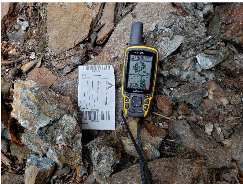
Photo 7.7. Semi-massive arsenopyrite and pyrite in a silicified carbonatized seam within sheared and altered mafic volcanics along the Blackwater Fault, photo by LLG, 2020.
