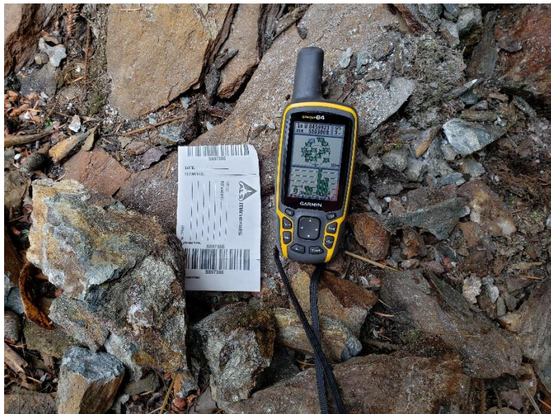
Photo 7.7. Semi-massive arsenopyrite and pyrite in a silicified carbonatized seam within sheared and altered mafic volcanics along the Blackwater Fault, photo by author.
