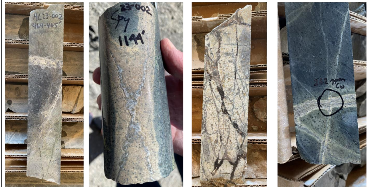
AC23-002: Drill core showing intensely and pervasively k-spar altered and well mineralized pyrite-chalcopyrite-k-spar stockwork veining. Hydrothermal breccias contain extensive replacement of primary mineralogy and texture by chlorite, epidote and calcite with ubiquitous pyrite stockwork veining and disseminated chalcopyrite+/- magnetite.
