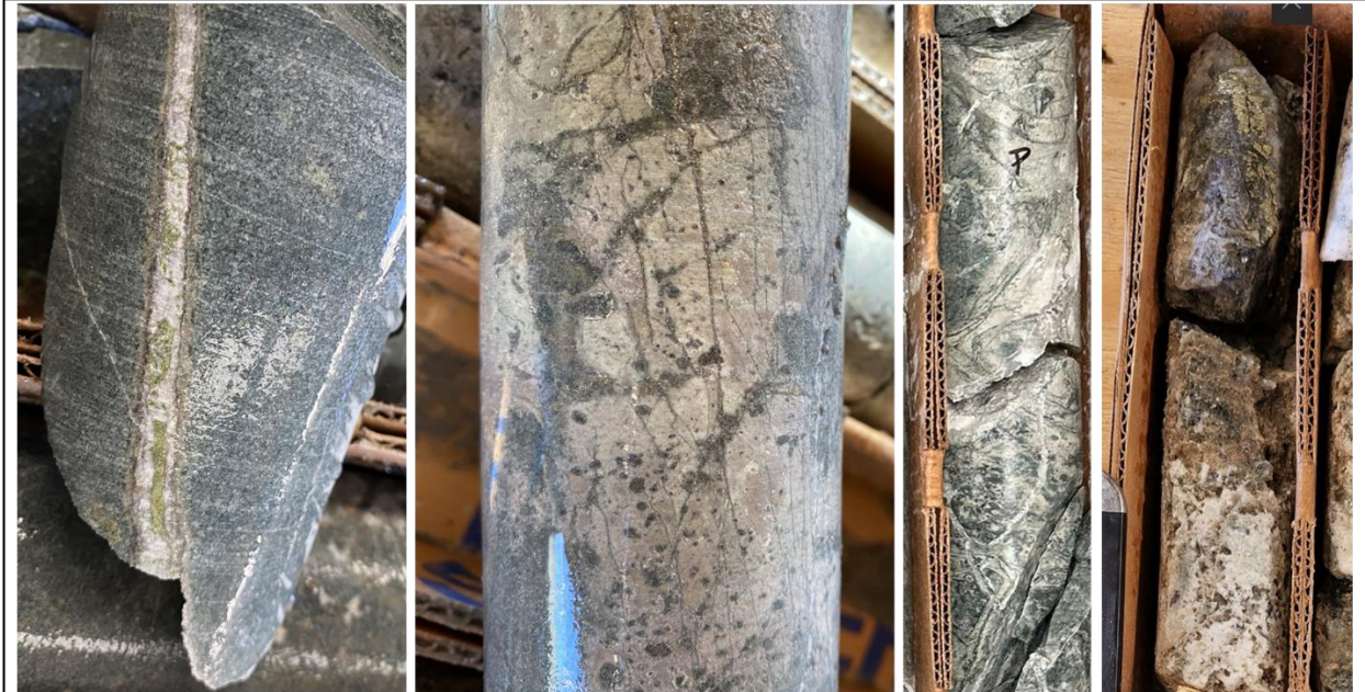
AC23-005: The Last Chance vein characterized by coarse grained masses of chalcopyrite and chalcopyrite veinlets with some 5 ft intervals displaying over 1% Cu assays. Pervasive phyllic and propylitic alteration is present throughout the drill hole with extensive pyrite +/- chalcopyrite + magnetite stockwork veining.
