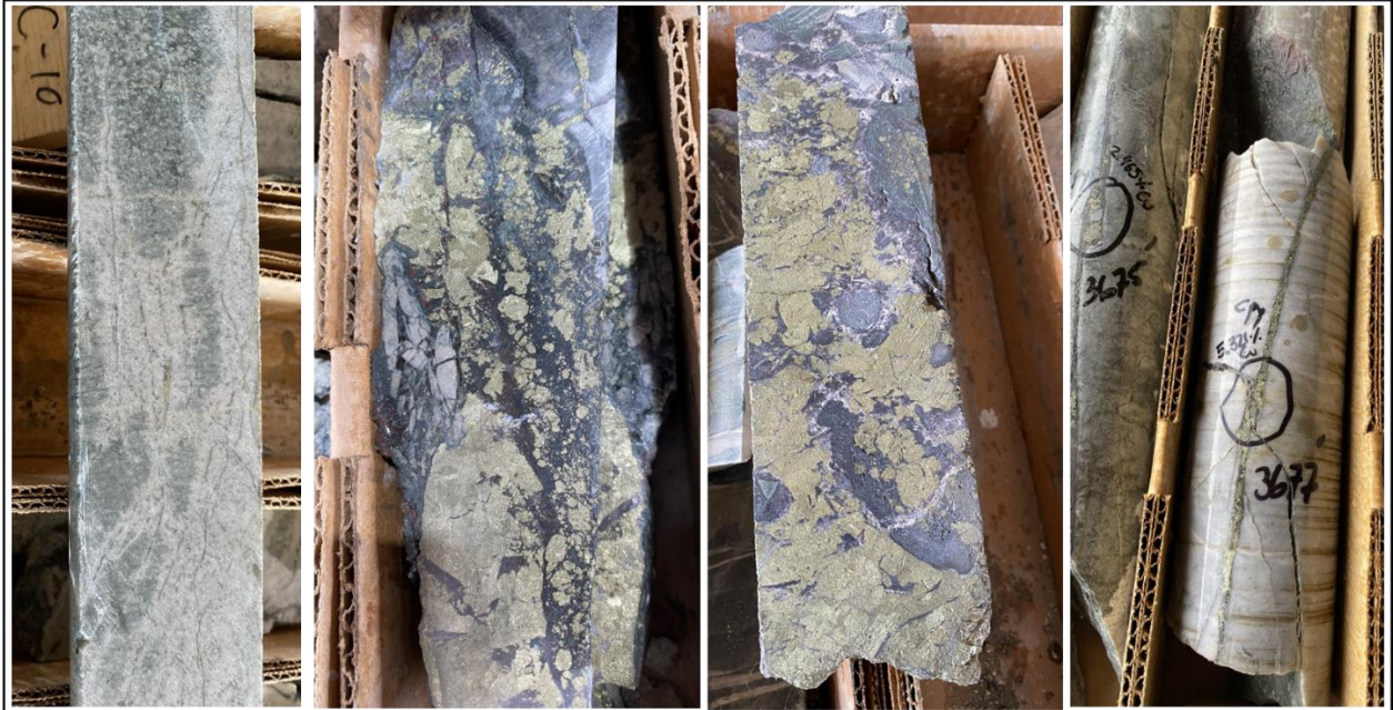
AC23-004: Mineralized intervals typically contain common, thin, irregular chalcopyrite veinlets with irregular, seemingly arbitrary, zones with chalcopyrite concentrations greater than 50-percent of the core volume.
