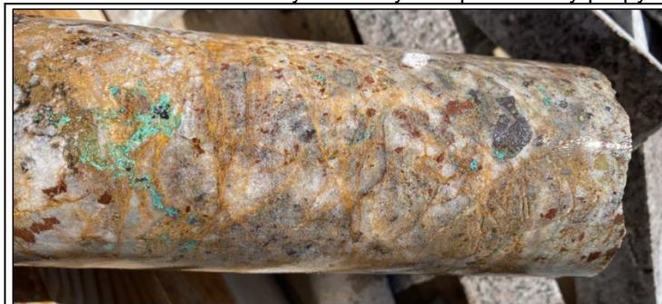
AC23-001: Copper oxide and sulfide mineralization (azurite, malachite, chrysocolla, chalcopyrite), pyrite and magnetite mineralization in highly silicified rock.
