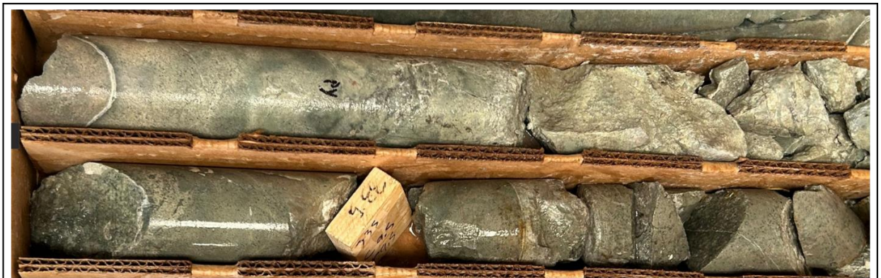
AC23-003: Clay-altered feldspar porphyry with epithermal-style quartz vein stock work containing 40ppm Ag and 0.5ppm Au.
