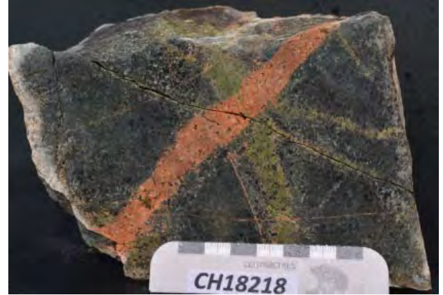
Figure 41: Photo CH18218 potassically altered veinlet in Monzodiorite from the Coho Zone Sawn sample from Ron Bilquist's 2018 exploration of the Coho Zone showing strong potassic alteration along a planar structure. Epidote alteration crosses the potassic zone along fine filaments sulphide mineralization along fractures Cu=73ppm 403645E; 6120491 N.
