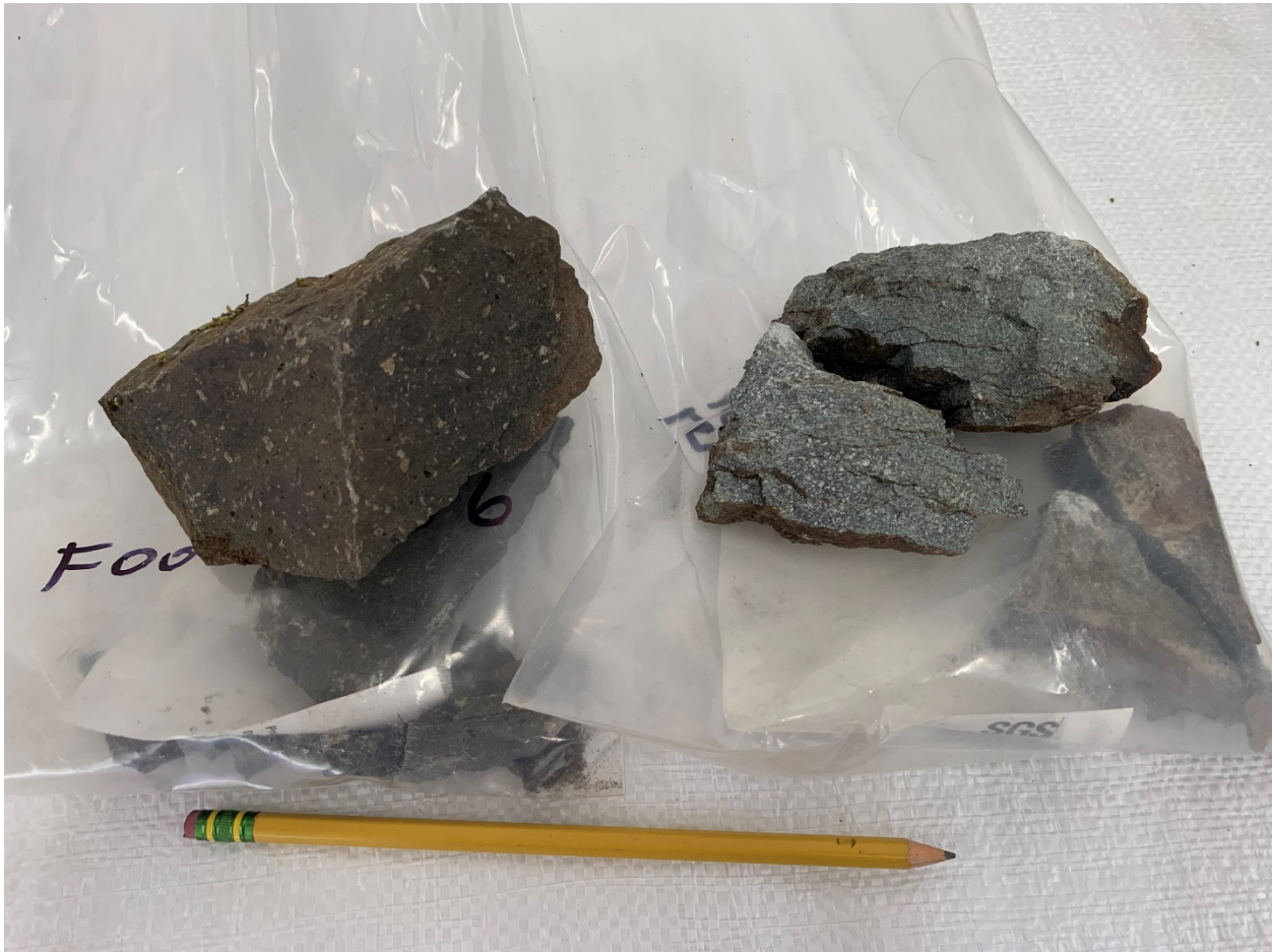
Figure 12.1 – Rock samples the author collected on the July 18 site visit. Outcrop consists of the Endako Group grey, brown, maroon green, phyrlic trachyandesite
