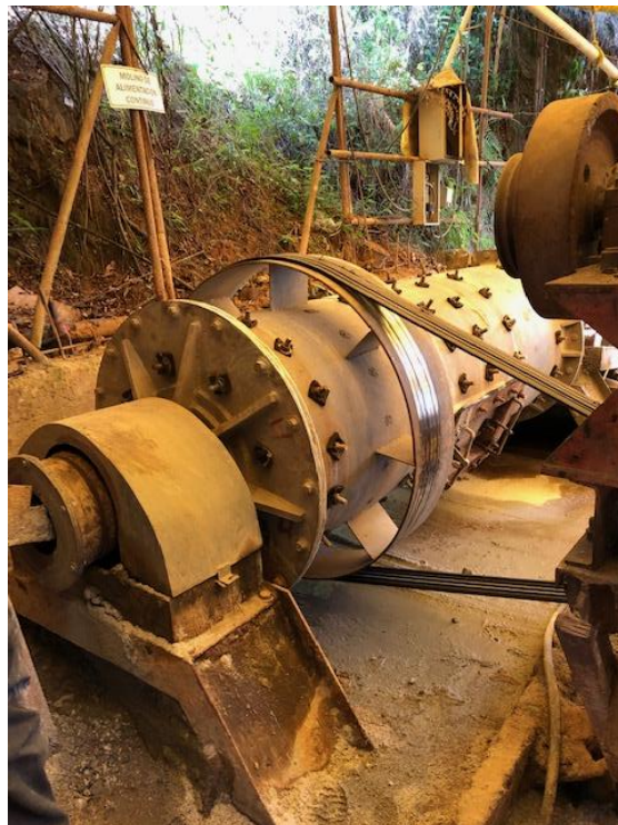
Ball mill at Purimac Mine
