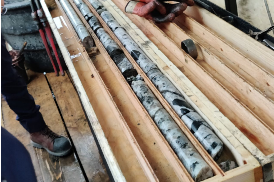
Photo 1: Spodumene-bearing pegmatite being actively cored in CV22-041 during site visit to drill rig
