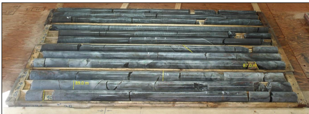
Figure 1.6 Gold Mineralization in Quartz-Carbonate Veins in Hole SD-19-06
