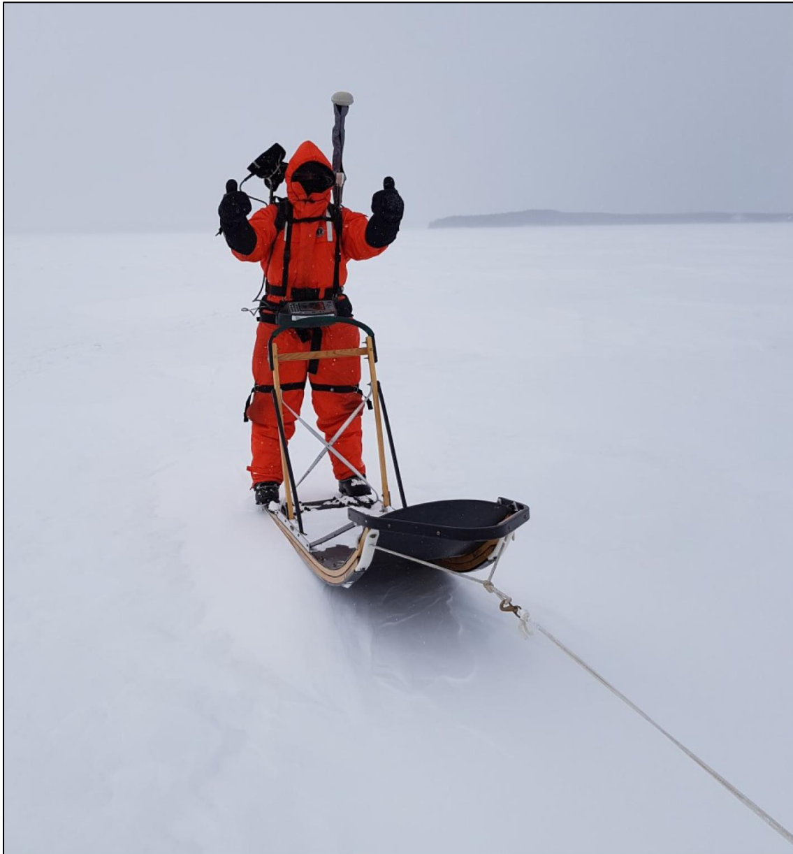
Figure 9.11 FN Instrument Operator on DogMAGTM Non-ferrous Dog Sled at Fishtail Bay
