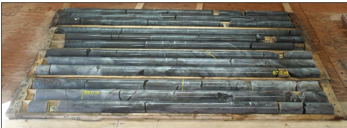
Figure 7.7 Gold Mineralization in Quartz-carbonate Veins in Hole SD-19-06
