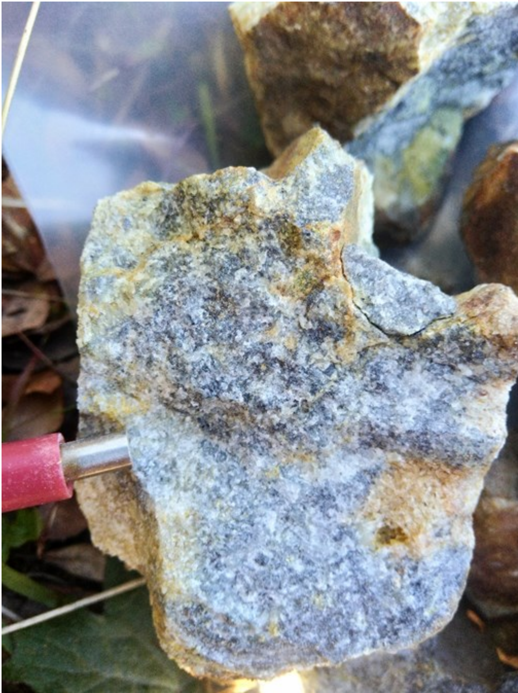
Sample C0216025: Strongly silicified and veined quartz feldspar porphyry with vuggy scorodite from east of Ed grid: 591 g/t silver & 10.2 ppm Au
