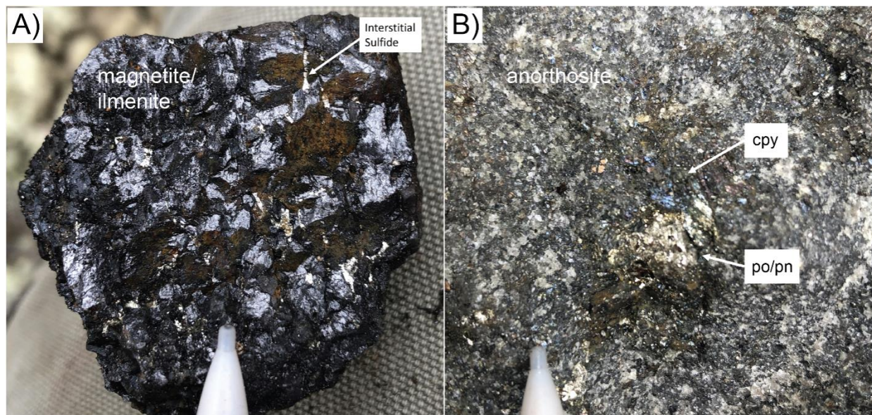
Figure 8. Examples of Ni-Cu enriched samples with interstitial sulfides, locally with ISS/MSS segregation (chalcopyrite, cpy, and pyrrhotite-pentlandite, po/pn).
