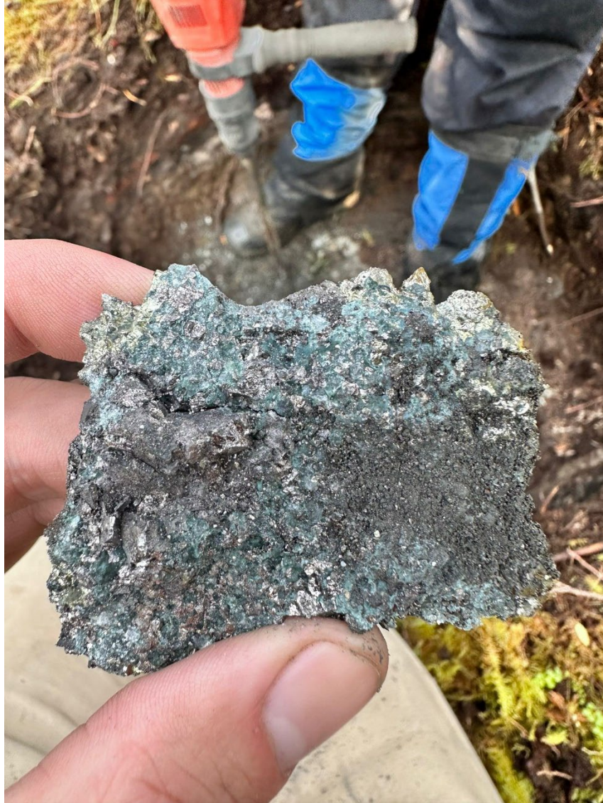
Figure 1. Grab sample 344465 showing intercumulate texture of pyrrhotite and/or pentlandite with chalcopyrite and silicate minerals.
