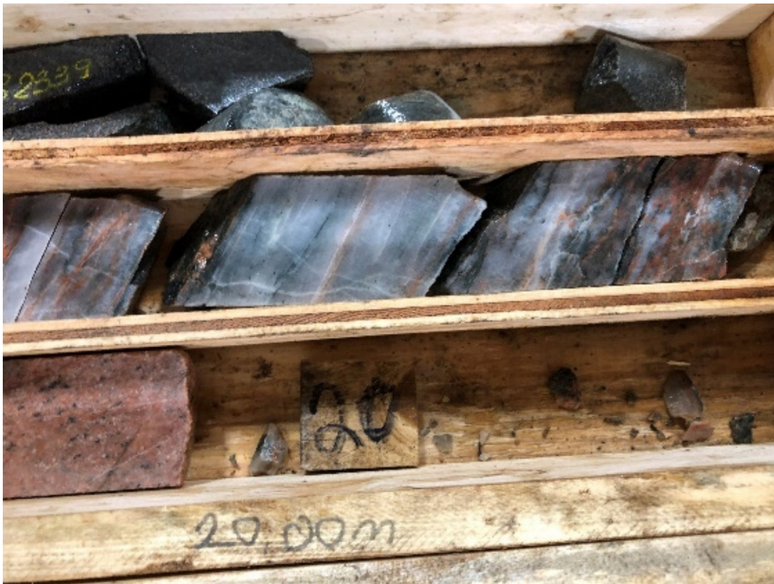
Figure 26. The silicified shear zone in hole UTG-21-005 at 18.50 m. This interval is representative of the highly strained and banded silicification that is consistent with the gold-bearing No1. Zone.
