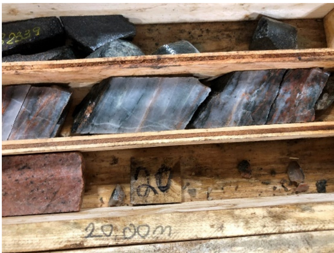
Figure 26. The silicified shear zone in hole UTG-21-005 at 18.50 m. This interval is representative of the highly strained and banded silicification that is consistent with the gold-bearing No1. Zone.
