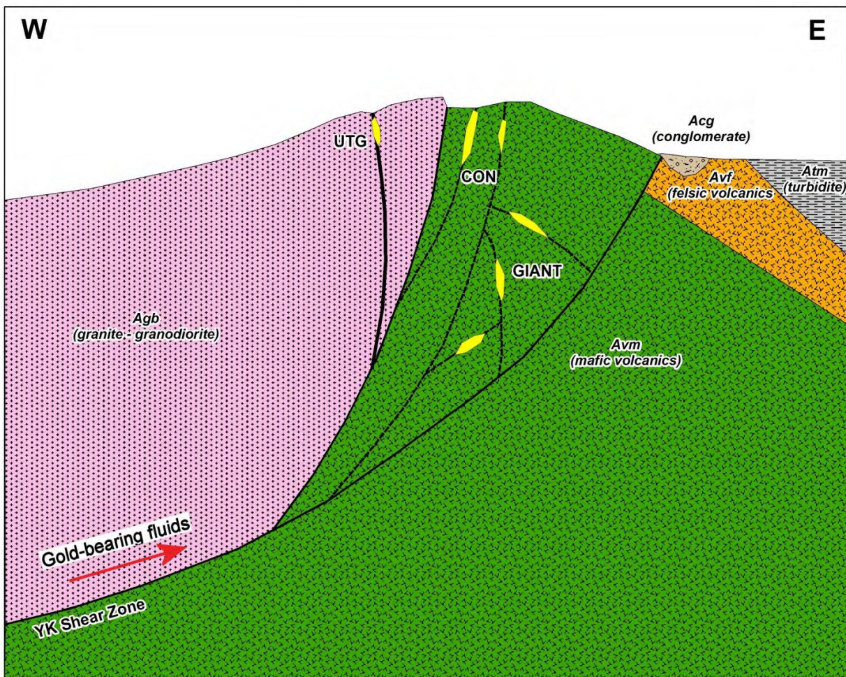
Figure 13. Conceptual model for Archean lode gold mineralization - Yellowknife Greenstone Belt (modified after Power, 2016)
