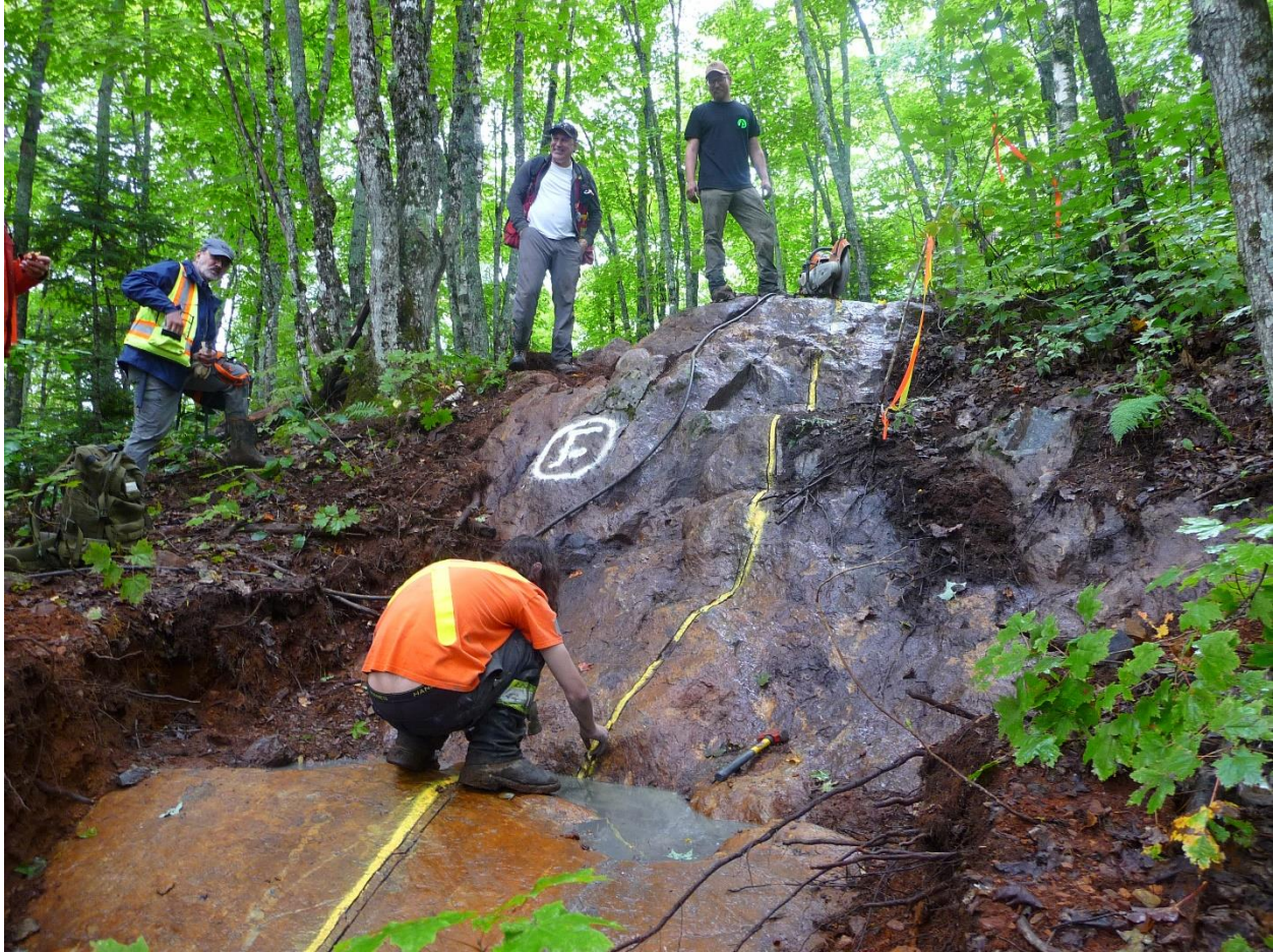
Photo of the field crew cleaning and sampling massive sulphide exposure in Area F.
