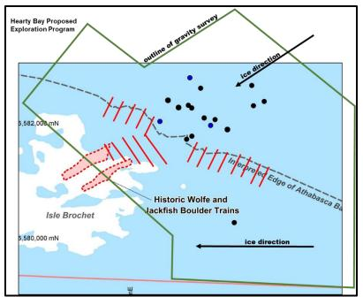
*Location Map of the Radioactive Boulder Trains.* The green line shows the extent of the gravity survey, the parallel red lines will be drill fences to be completed along with any targets generated by the survey.
