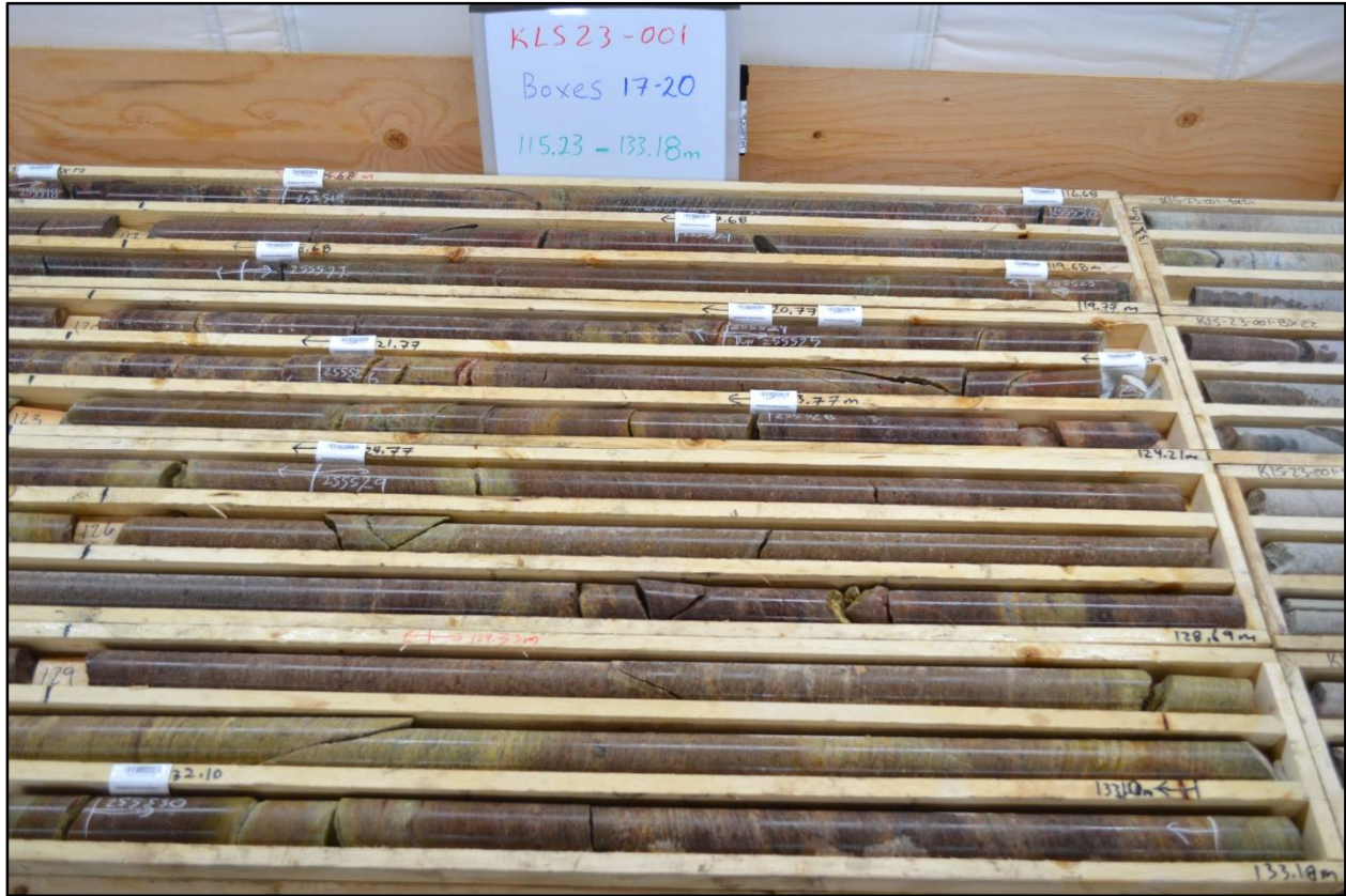
Figure 10: Pervasive epidote, hematite alteration, DDH KLS23-001, Boxes 17-20.
