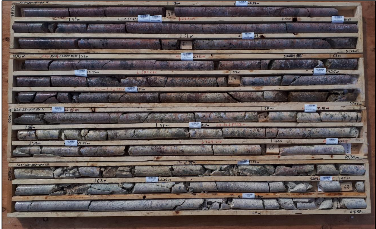
Figure 5: DDH KLS23-007, Core from Anomalous Zone (47.37 - 64.57m)
