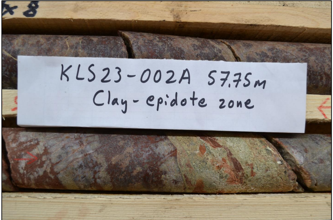
Figure 4: DDH KLS23-002A (57.75m depth) Clay-Epidote Zone
