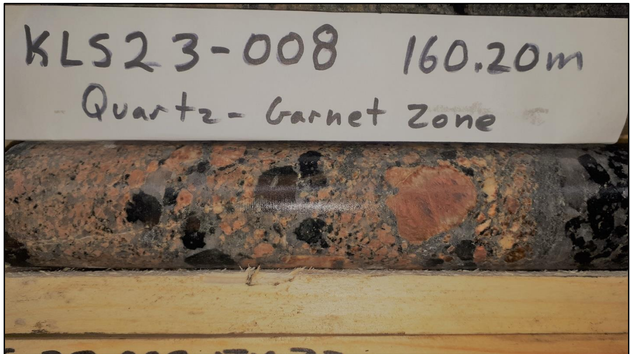
Figure 7: DDH KLS23-008 (160.2 m depth): Quartz-garnet zone
