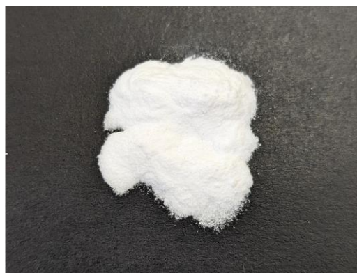
Photo 13-1: Photograph of Battery-Grade Lithium Carbonate Sample (4063-119-3), Sample Spread over Approximately 1 in. Diameter
