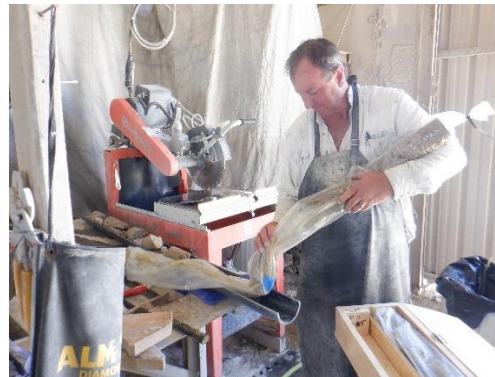
taking out the first 5 ft core from the core box and putting the core into a PVC pipe cut in half
