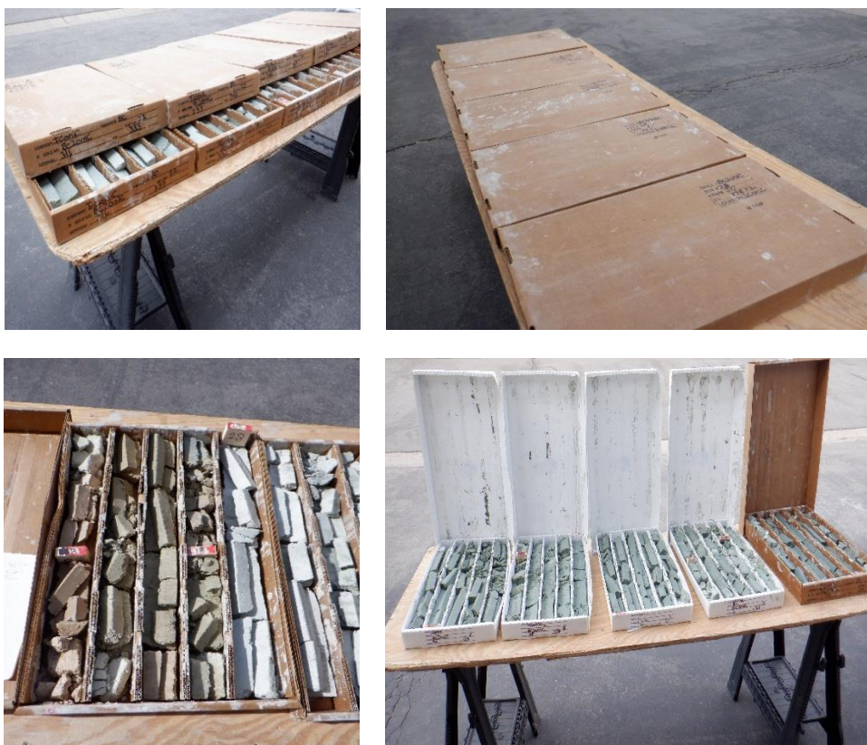
Photo 11-2: Core Box Labeling (upper photos), Core Sample from BC2001C (lower right) and from BC2002C (lower left)
