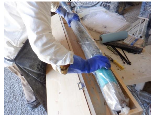
1/4 core into a sample bag for assaying and half core plus 1/4 core return to the core box
