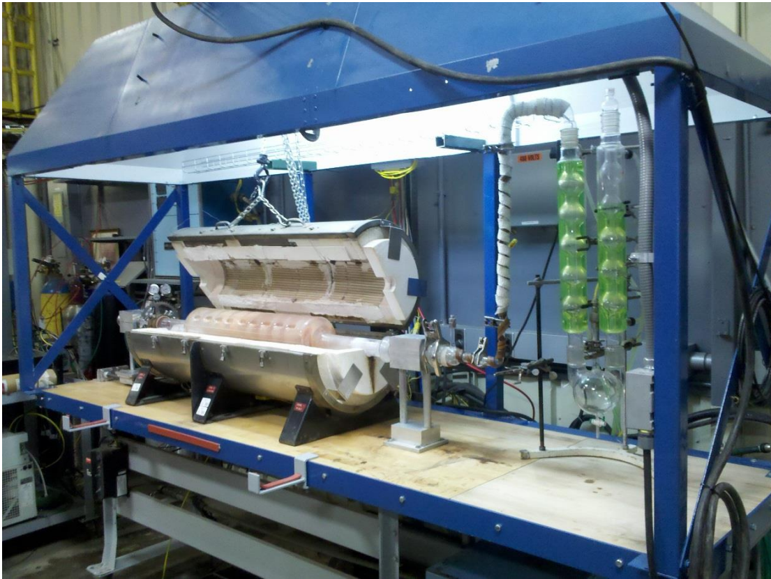
Figure 13-5: Batch Rotary Kiln System (7 in.)
