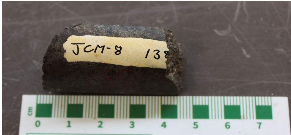
Figure 1 – Mal Lake Drillhole JCM-8 @ 138 feet (42.06m) split core, mineralized quartz diorite; pXRF scan @ 138.75 feet (42.29m): 21,146ppm Ni, 1,322ppm Cu, 1,480ppm Co; Note historic assay interval 38.98-43.19m in Table 1
